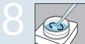
Immediately mix using a brush applicator until gel is homogeneous.
